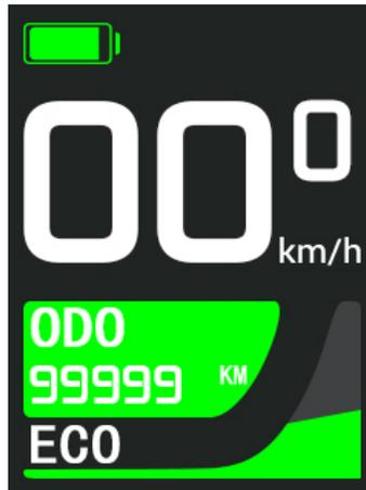
Real-time speed and Odometer display
